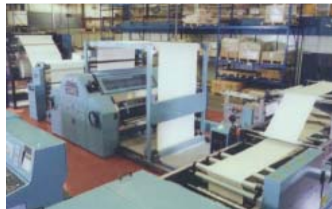
This Timson T48A bookpress is similar to others supplied to Australian book printers by JL Lennard Graphics.
