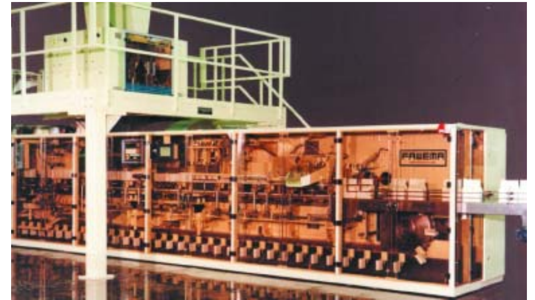
A modern high-speed packaging machine for products such as flour, sugar and pet food, manufactured by Fawema in Germany.
